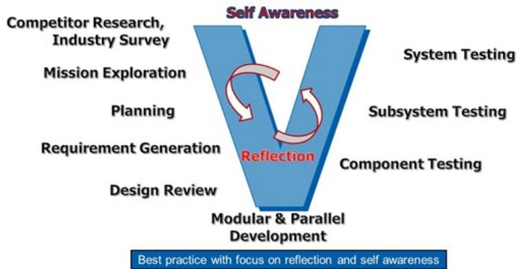
Figure 2. Team Inspiration Systems Engineering V Process for RoboSub
