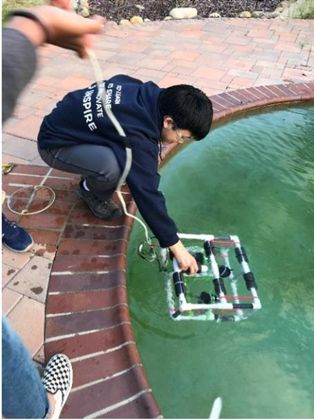
Figure 4. Simple PVC Robot with Remote Control
