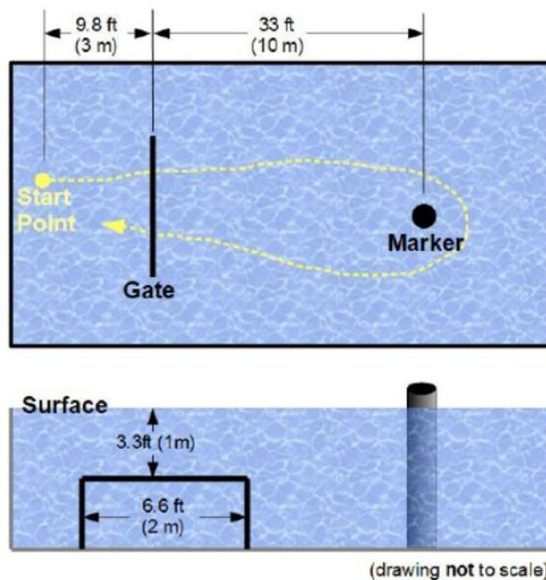
Figure 1. Vehicle Pre-Qualification Specification
