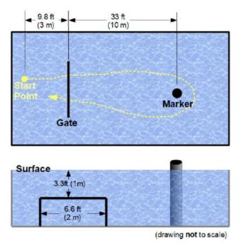
Figure 1. Vehicle Pre-Qualification Specification
