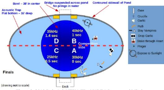
Figure 3. 2019 RoboSub NIWC TRANSDEC Layout and Mission
