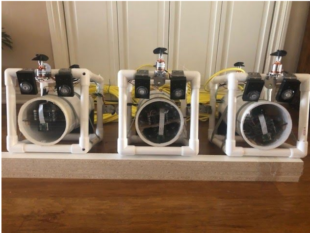
Fig. 7. Prototype ROVs developed in collaboration with Porpoise Robotics.
