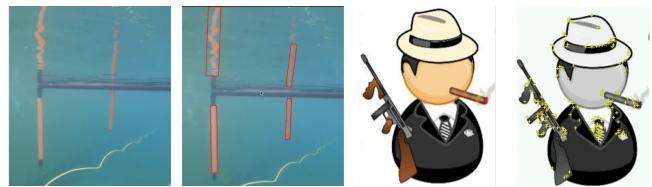
Fig. 3. OpenCV processing a frame of the gate; Vuforia identifying features of the bootlegger.
