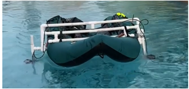
Figure 8. The float tube with thruster attachment mounted
