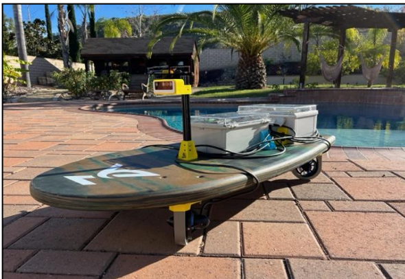
Fig. 1. Alpha Design with Holonomic Thrusters
